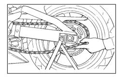
6. Push the wheel forward, and then remove the drive chain from the rear sprocket.
